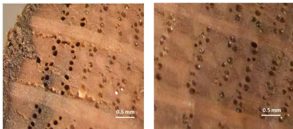
**Figure 3.** Cross section of oak wood excavated in archaeological works in the prehistoric settlement in Ropotamo River estuary
