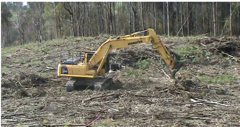
Figure 1. Excavator clearing harvesting residue into windrows
