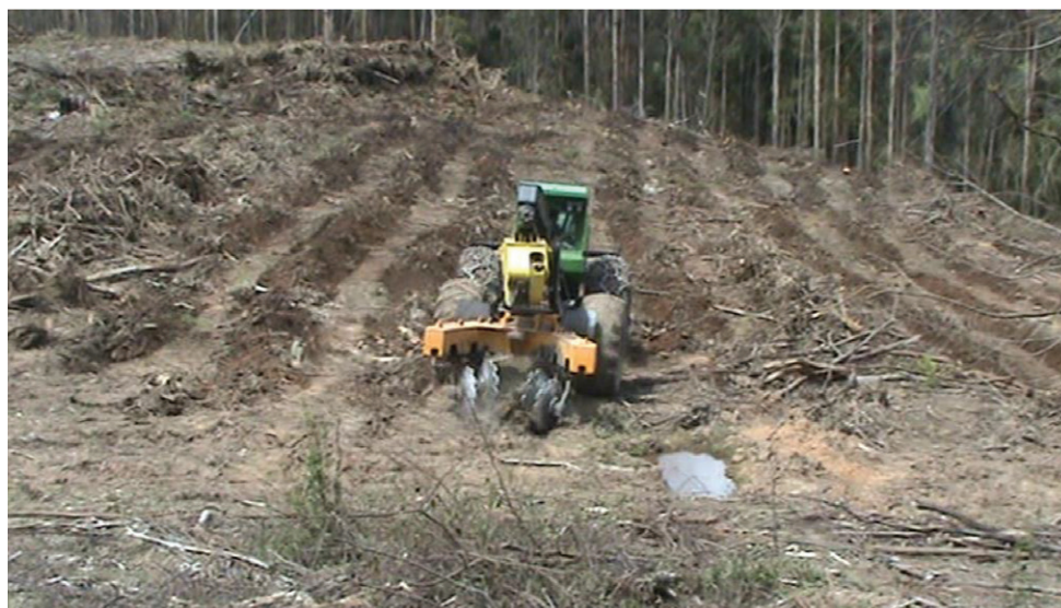
Figure 2. Skidder-mounted plough ploughing furrows
